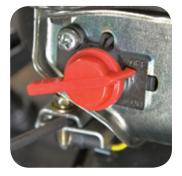
1. Turn engine/motor to Off position.
