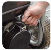
8. Gas Pressure Washers Pull starter cord until pump protector fluid is discharged from pump outlet. (DO NOT START ENGINE)
